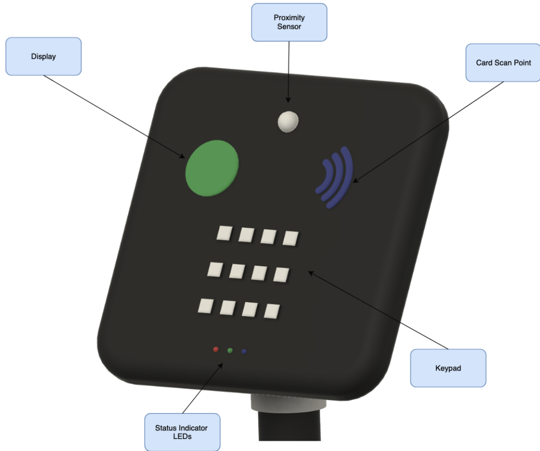
Figure 2.1 Rendering of SCAN Kiosk Prototype
